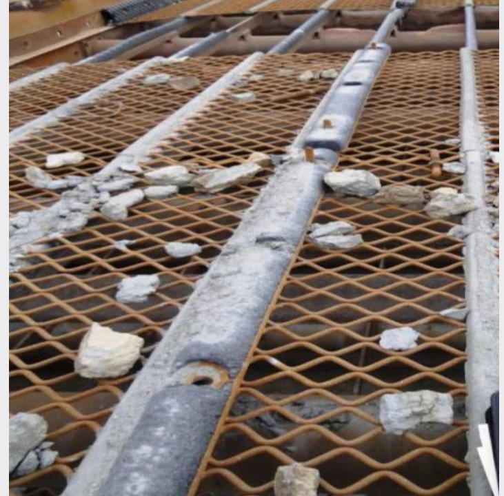
* Image of competitor's 2" wobble wire on top deck of secondary scalping screen
