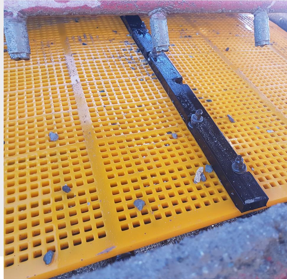
*\*Image shows competitor's side-tensioned urethane media that required a center bolting strip to hold the media in place adding extra hardware and weight on the deck.*
