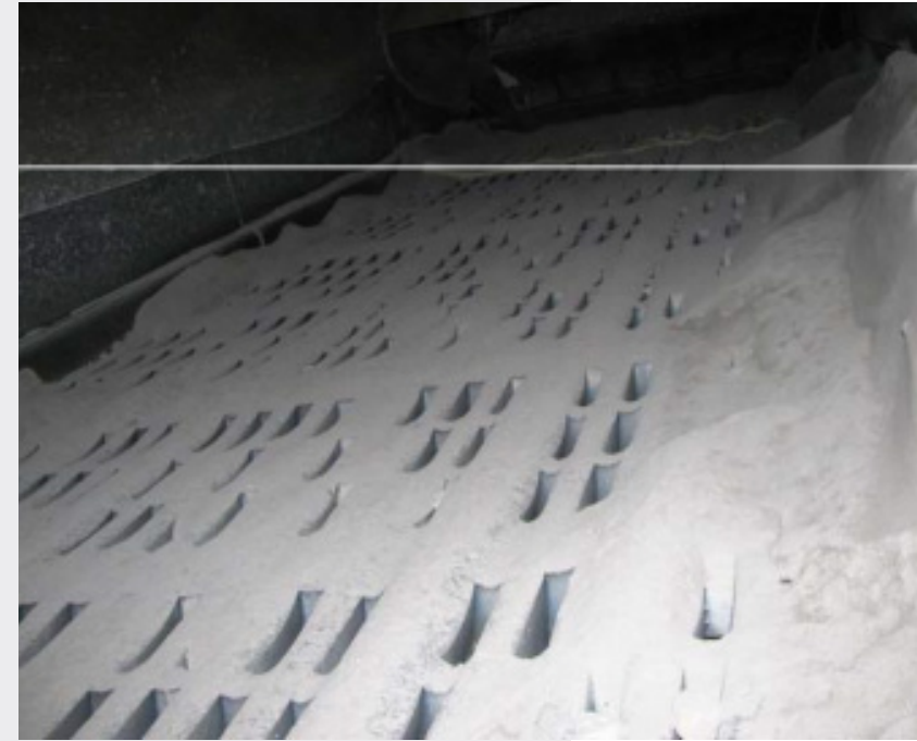
* Image shows competitor bolt down rubber showing pegging/plugging and blinding.
