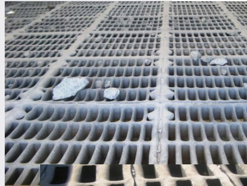
* Image shows Polydeck's high open area Maxi Slotted panels with 36% open area.
