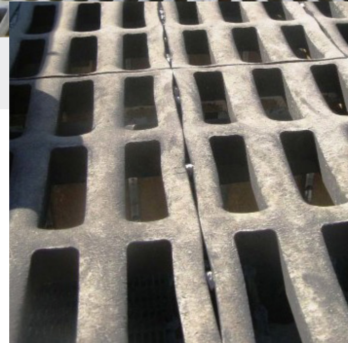
* Image shows Polydeck's heavy-duty panels installed in feed zone to optimize wear life.
