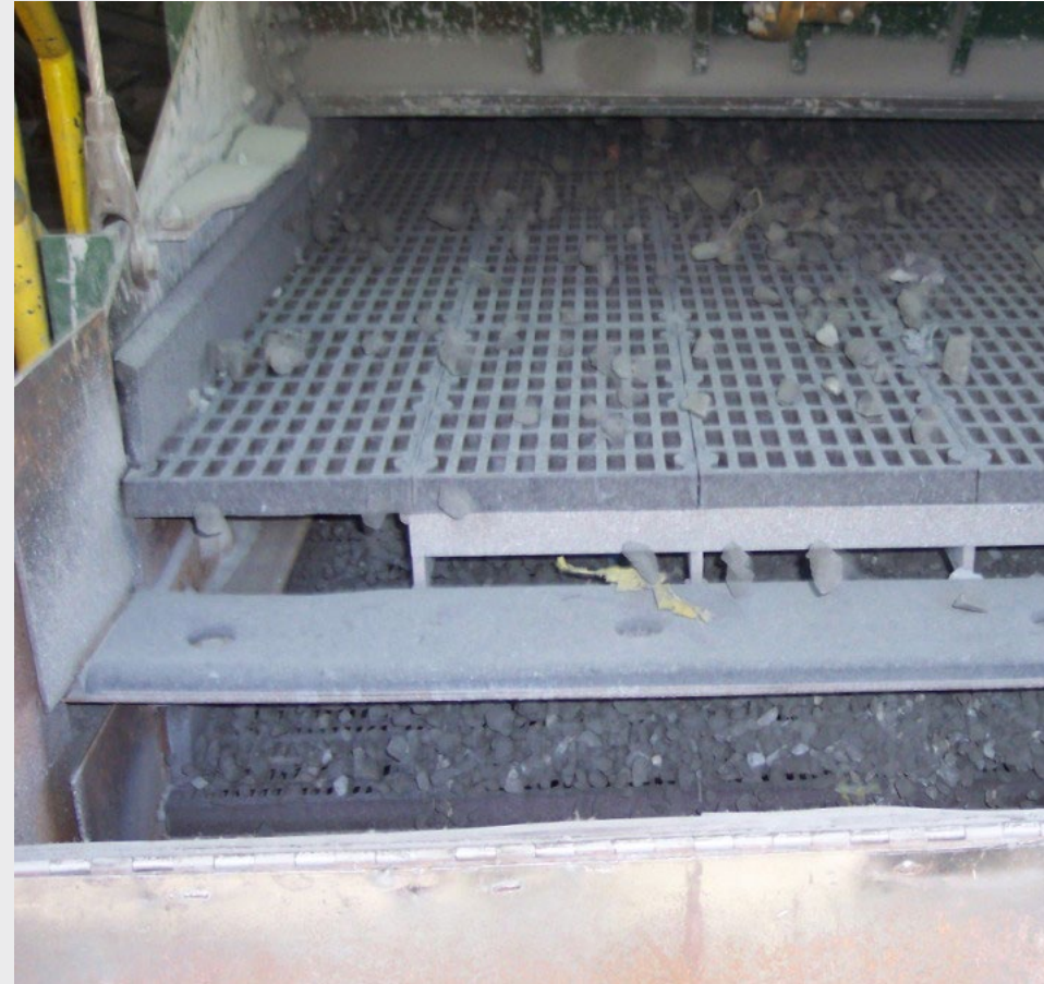
* Polydeck's Flexi designed rubber panels decrease blinding and plugging issues.
